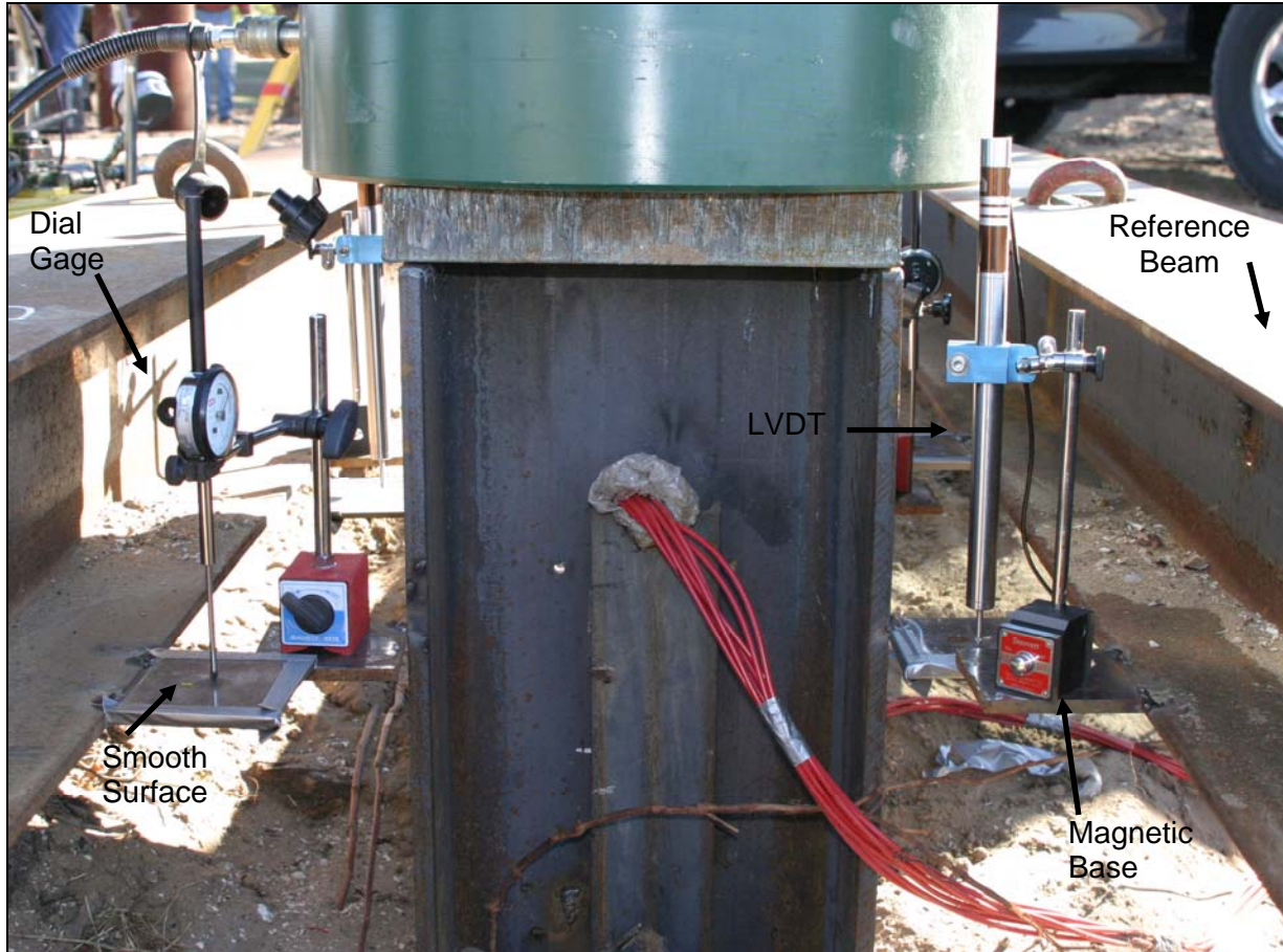
Figure 9-65. Load test movement monitoring components (FHWA, 2006a).
